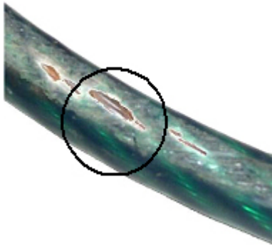
Figure 5. Damaged plastic coated wire rope.
